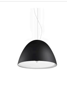
Suspension lighting fixture for interiors, with direct light emission. Turned pickled sheet metal structure in metallized grey polyacrylic paint. Lampshade in black decorated blown glass. Diffuser in modelled frosted glass. 2m (78,7") long steel suspension cable. 2,2m (86,6") long power cable in transparent PVC. Power canopy with galvanized sheet metal ceiling bracket and pickled sheet metal
